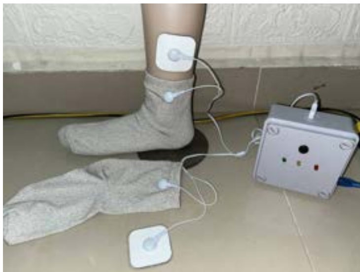
Figure 3: Electro Socks Massage prototype
