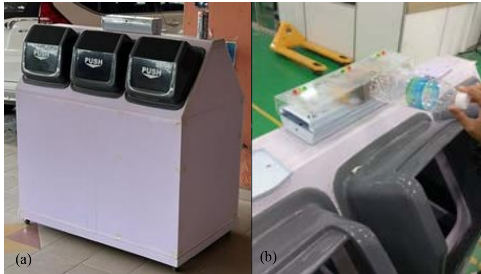
Figure 5: a) The developed Smart 3R Bin, b) Object from plastic was detected and yellow LED lights up
