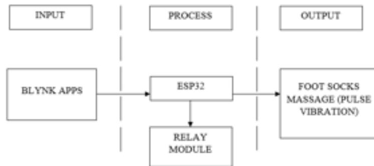
Figure 1: System Design and Architecture
